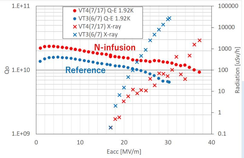
**Eacc** for reference measurement was limited by F.E.
