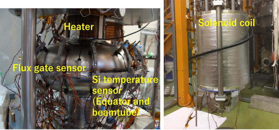
Flux gate sensor, Si temperature sensor, heater and solenoid coil were used.
