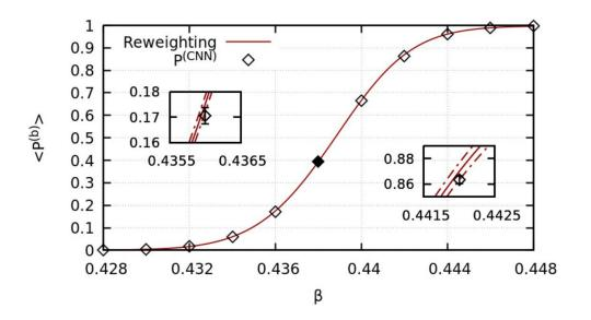
Training was conducted below  $\beta$ =0.41 and above  $\beta$ =0.47 **Red line**: obtained using reweighting from a single dataset at  $\beta$ = 0.438 (filled point) **Empty points**: Actual calculations of the neural network on independent Monte Carlo datasets.
