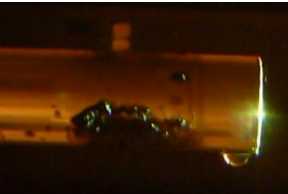
MINOS NT-01 target water leak (FNAL)
