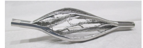
Iridium target tested at CERN's HiRadMat facility
