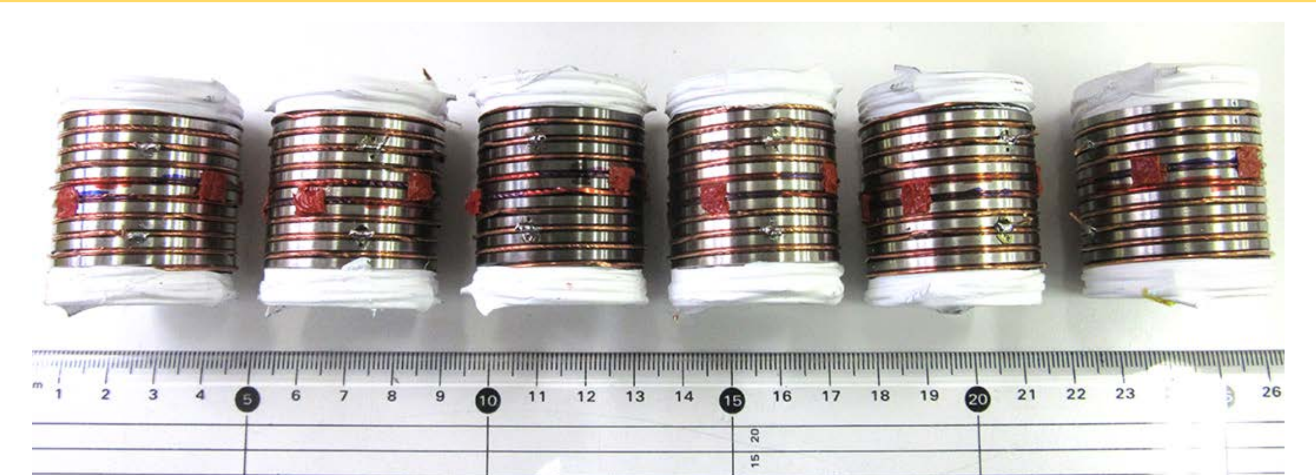
NbTi short samples on Ti-6Al-4V alloy barrel.
