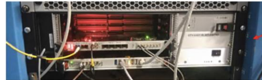
ELMA VME crate + MEN A25 CPUs + CTRP module + VFC-HD + FMC-1000
