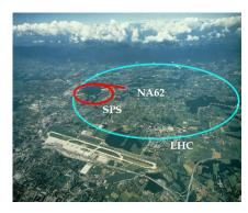
NA62 is located at CERN in the *North Area*, exploiting a 400 GeV/c proton beam extracted from the SPS accelerator.
