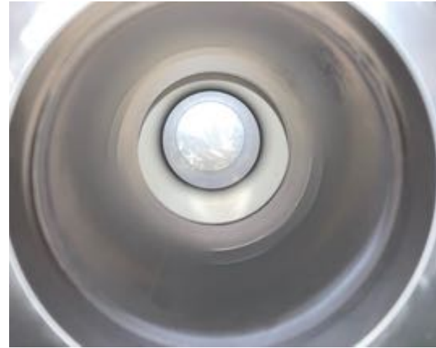
After coating: Metallic luster is lost. All of the inner surface is covered by Nb 3 Sn layer.
