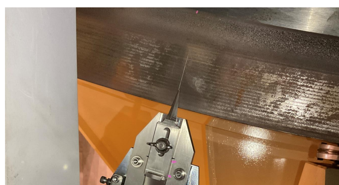
The marking indicating the origin position of the rotating gantry
