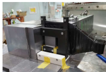
Photograph of ^{208}\text{Pb} target, collimators and shielding blocks
