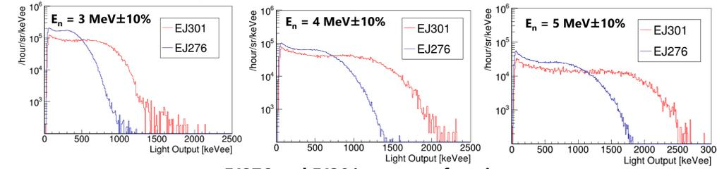
The experimental results show that EJ301 emits more light output than EJ276. In the future, the response function of EJ276 will be calculated by SCINFUL and compared with experimental results.
