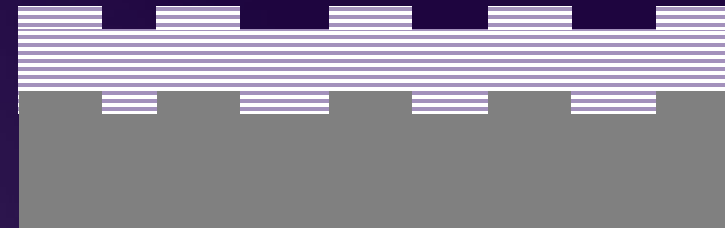
Mo/Si multilayer on relief substrate
