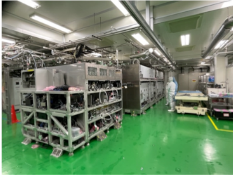
Fig.1 27kW Driver CO2 Laser System ( Gigaphoton
