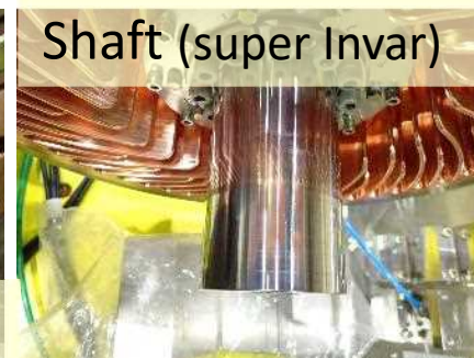
Photos after 100-times hard-landing tests.
