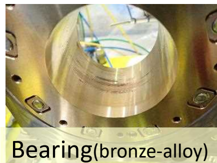
Photos after 100-times hard-landing tests.
