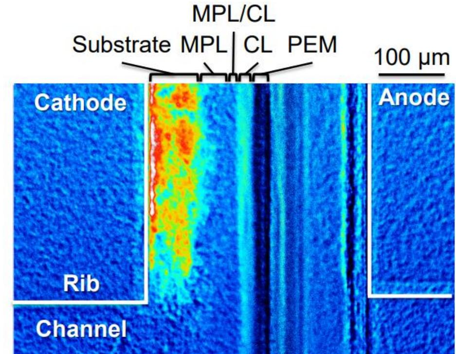
**Water distribution in the cell cross-section observed by synchrotron X-ray radiography\***
