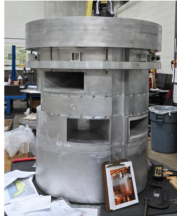
The Lower IRP, which contains the moderators and reflectors, is the last major component before final assembly.
