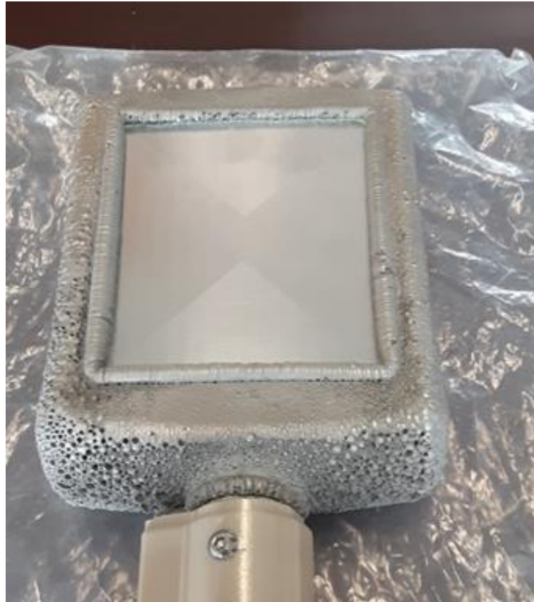
Initial testing had good adhesion, but excessive porosity
