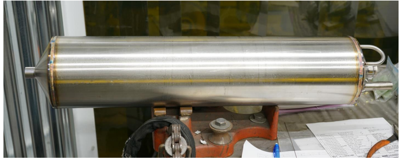
Welded 10-liter iron oxide catalyst bed
