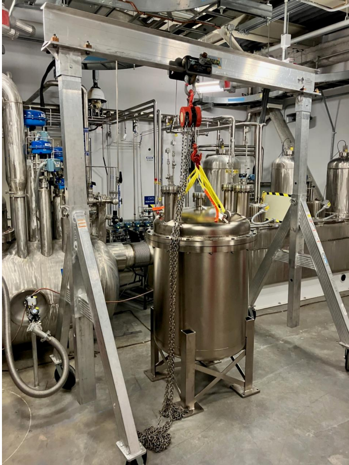
Vacuum vessel holding three catalyst beds
