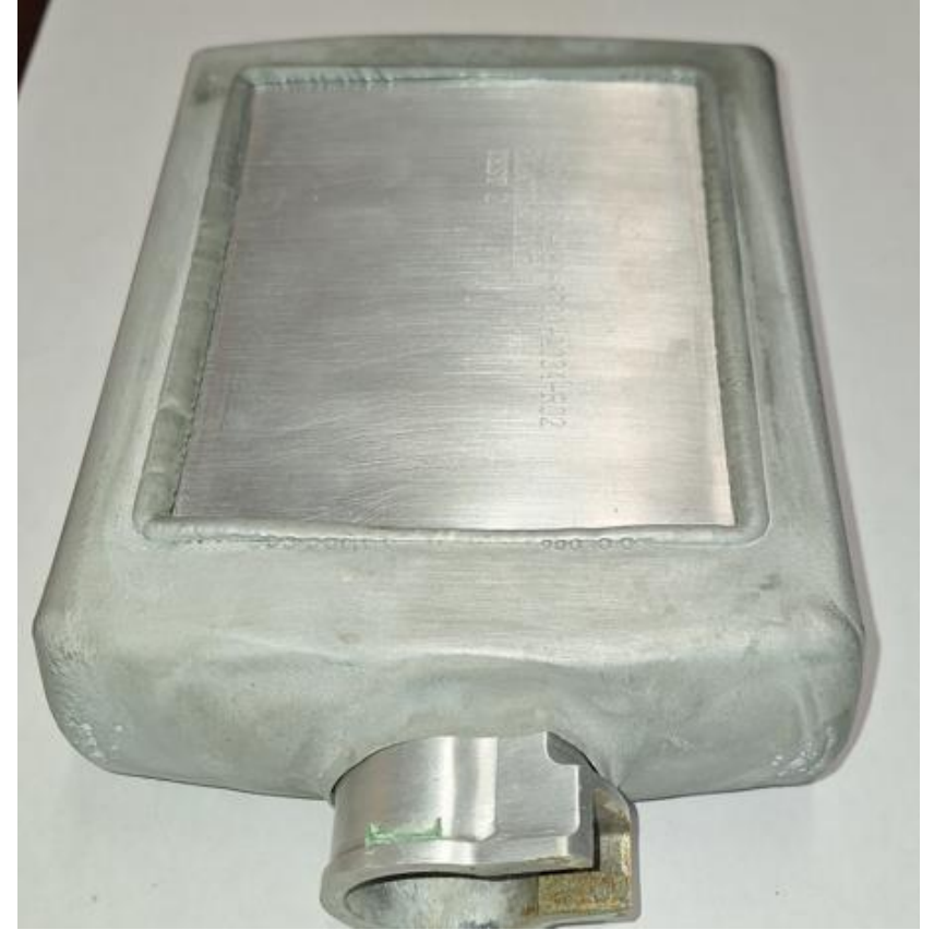
Addition of circulation and agitation system in the electrolyte bath resulted in good adhesion and density
