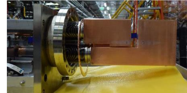
Static jaws made of Glidcop AL-15 are used in Low Power Charge Selector
