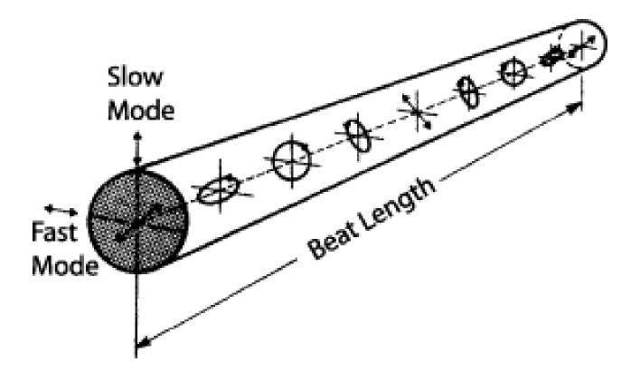
Fast mode / axis: relatively low refractive index Slow mode / axis: relatively high refractive index
