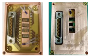
Fig. 6 Mounted film samples and thermometers: (left) without lid and (right) with lid.
