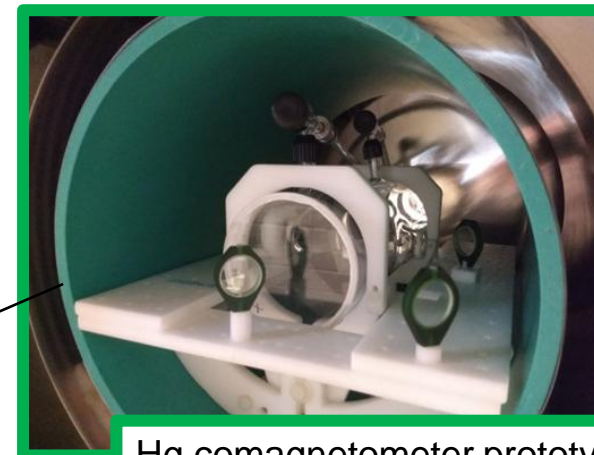
Hg comagnetometer prototype tested; preparing installation in MSR
