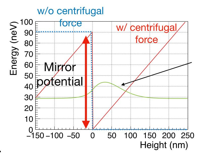
The quantum state of a neutron whispering gallery is confined between a mirror and the centrifugal force.
