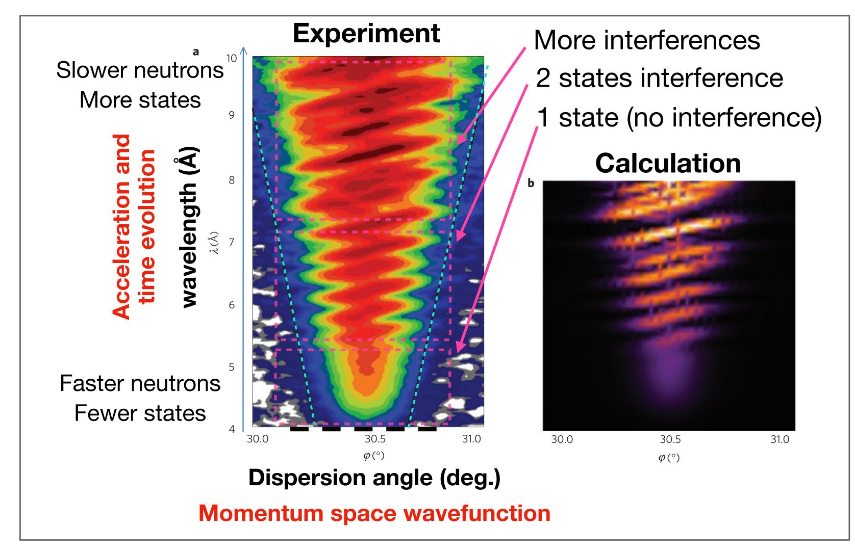
The interference fringe wavelength of the two lowest states is defined by  $(E_2 - E_1)t/\hbar$ . Therefore, we can measure the energy difference.
