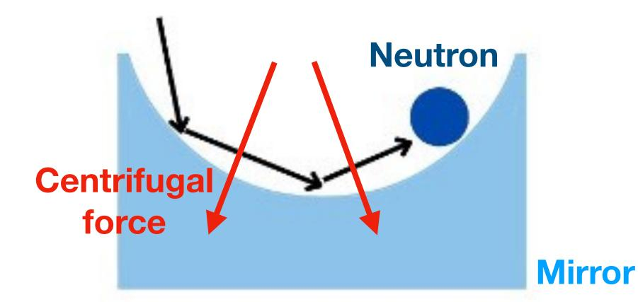
A neutron whispering gallery can be created using a cold neutron beam and a concave mirror.
