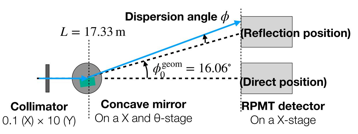
The angle span of the concave mirror can be determined by the neutron's dispersion angle.  $\rightarrow \phi_0^{\rm geom} = 16.06(2)^\circ$
