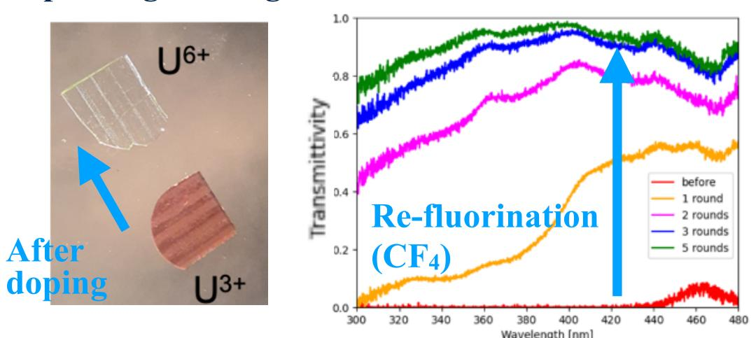
Establishing a method to control uranium valence enables new application for U:CaF<sub>2</sub>.
