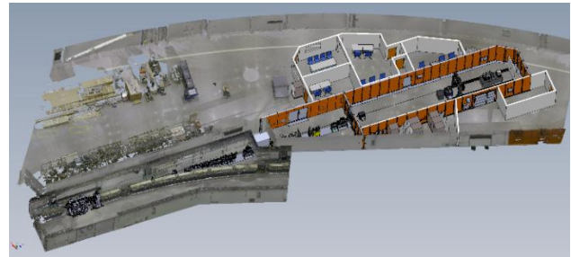
Figure 11: TomoWISE CAD beamline with meshed area in SolidWorks.
