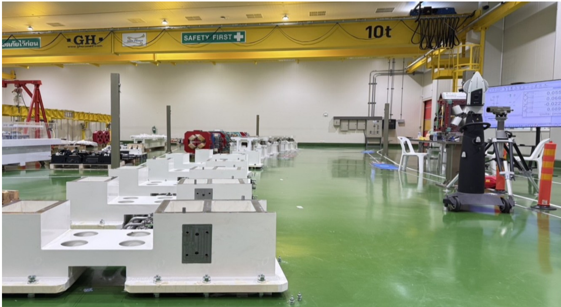
Figure 5: DTBA cell prototype and laser tracker setup in the pilot plant.
