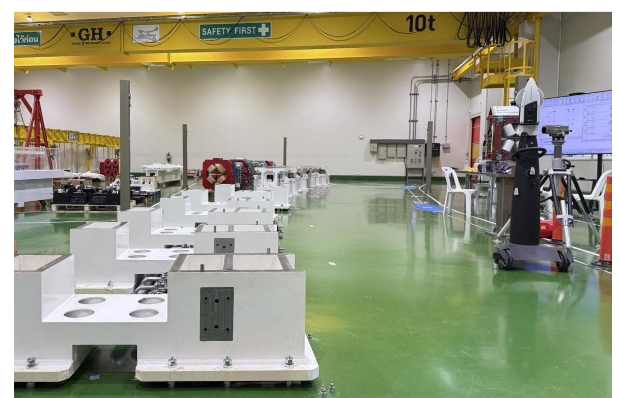
Figure 5: DTBA cell prototype and laser tracker setup in the pilot plant
