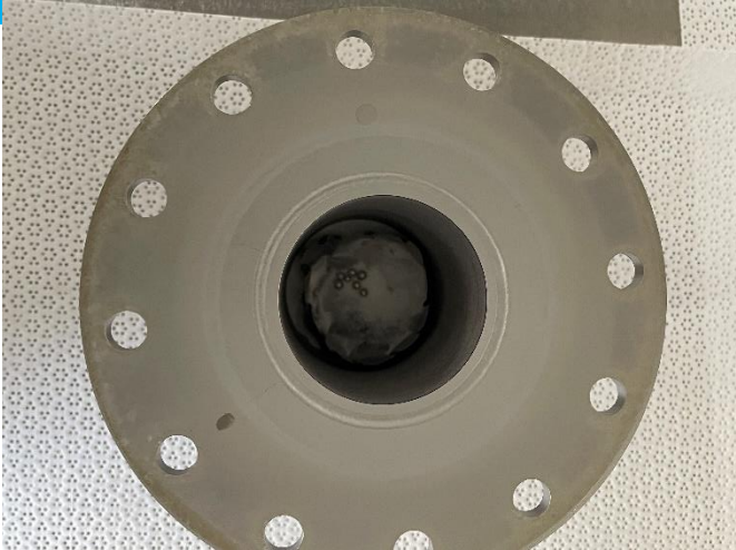
The Sn and SnCl 2 in the crucible
