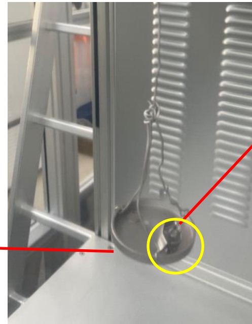
The second Sn source was put in the middle of the cavity.
