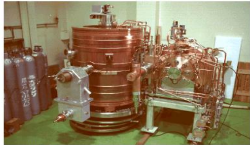
KEK ARES cavity, 509 MHz, 500 kV, 1.7 M \Omega
