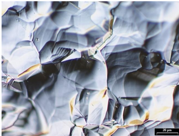
After 120 μm of BCP
