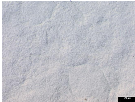
After 120 μm of EP
