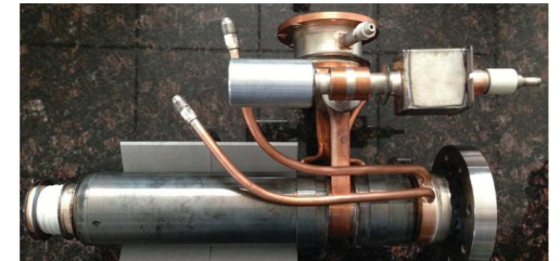
Compact X-band LINAC in Tsinghua University (2019)
