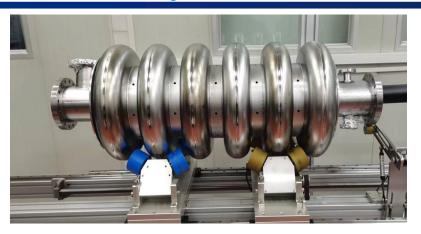
mechanical structure of prototype ellipsoidal cavity
