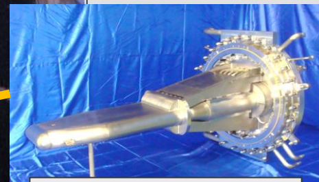
Neutron target Liquid metal, Mercury
