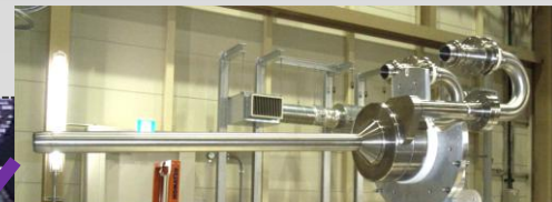
Neutrino target He-gas-cooled, fixed, Graphite
