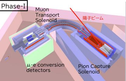
Target sensitivity: <10<sup>-14</sup> Proton beam power:3.2kW
