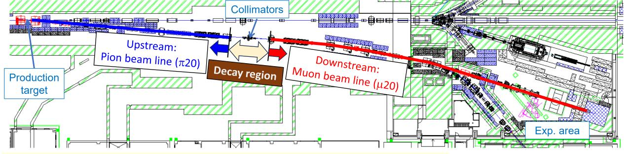
By changing the momentum settings downstream of decay region, only muons decayed from  $\pi$  are transported to exp. area.
