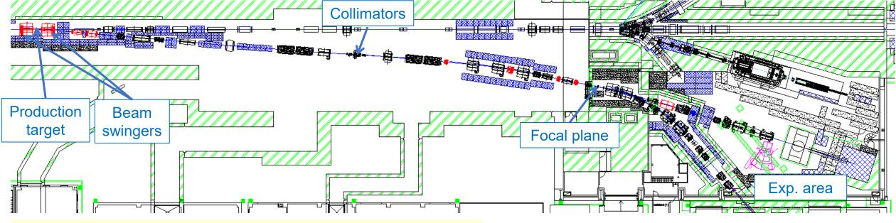
B-line is upgraded to a secondary beam line by adding a production target & some magnets
