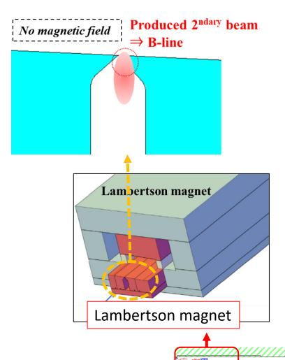
Test experiment **T106** has been carried out to measure positively charged secondary particles from the beam loss at the Lambertson magnet.
