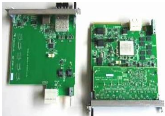
Cavity-field vector-sum in digital board #2
