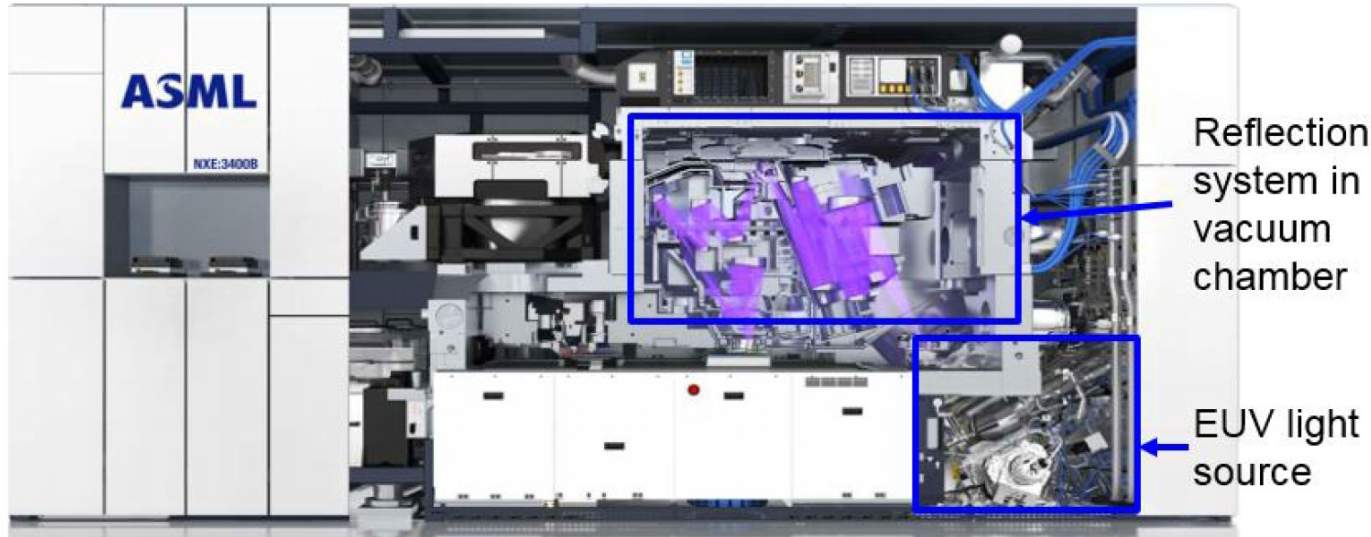
Figure 8. Internal structure of ASML NXE:3400B scanner. Source: ASML.
