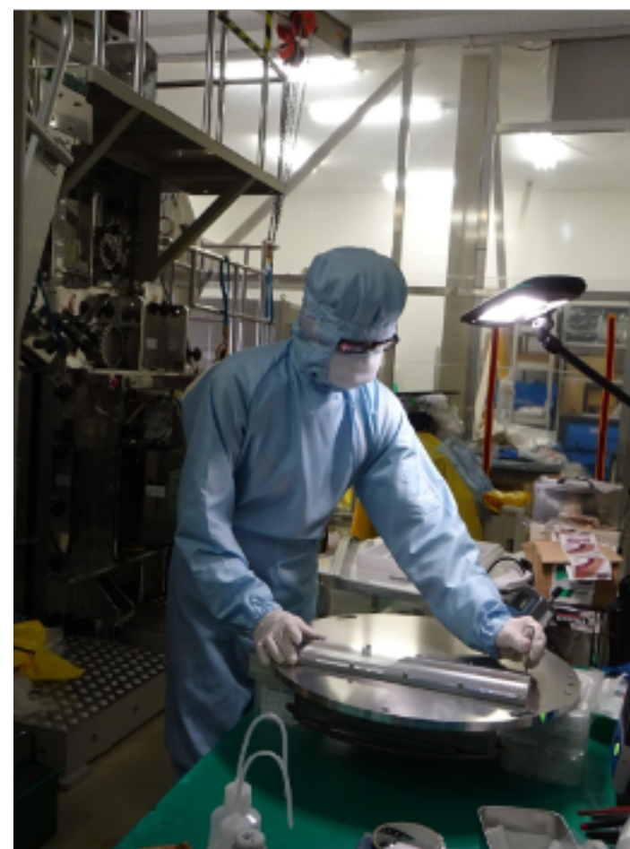
NiC/Ti supermirror was deposited on the substrate with 1D elliptic shape
