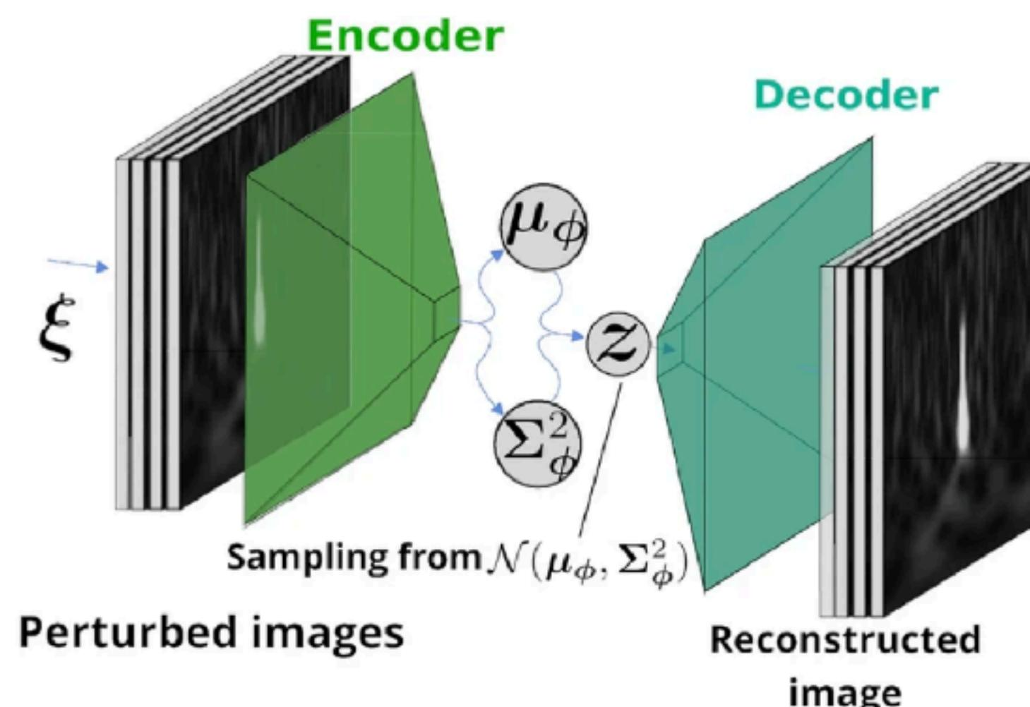
A generative encoder-decoder that learns a compact latent vector by reconstructing time-frequency glitch images
