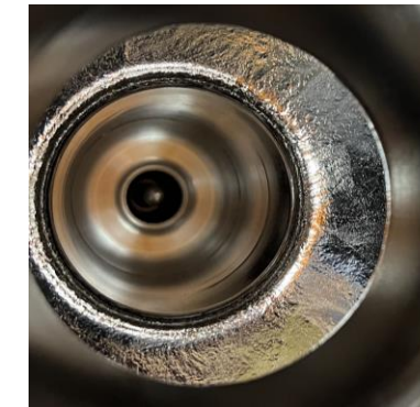
R18 & R18b HRRR MG Nb Tesla cavity manufactured at KEK-CFF
