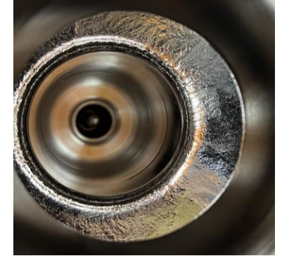
R18 & R18b HRRR MG Nb Tesla cavity manufactured at KEK-CFF
