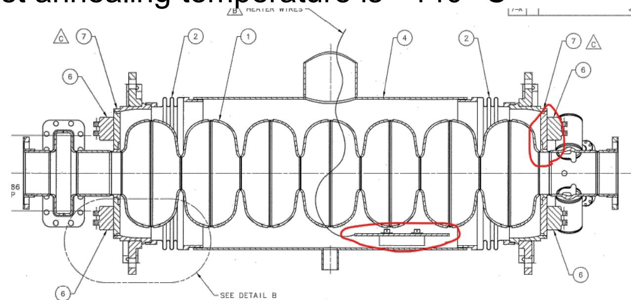
**Removal and reweld of Helium vessel is needed**
