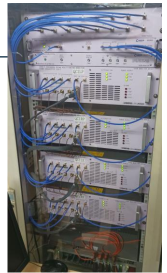
μTCA performs calculation on each channel of each BPM
