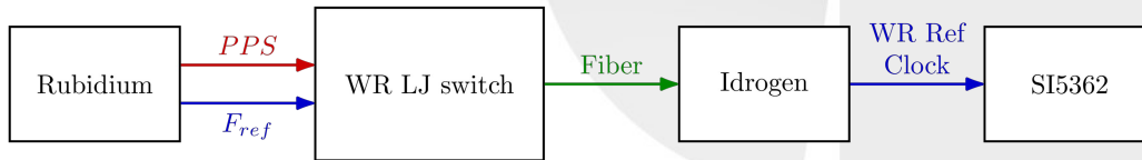
FPLL clock synthesis setup
