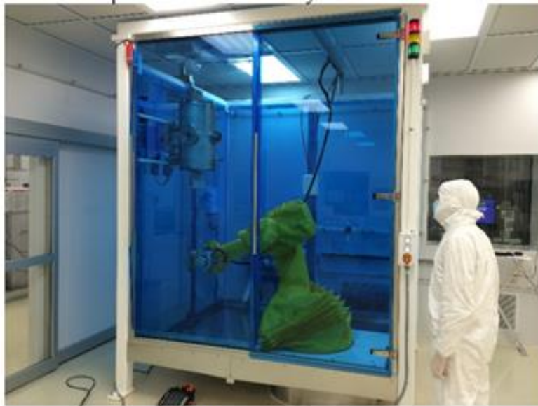
Figure 1: Robotic high-pressure rinse system, installed.
