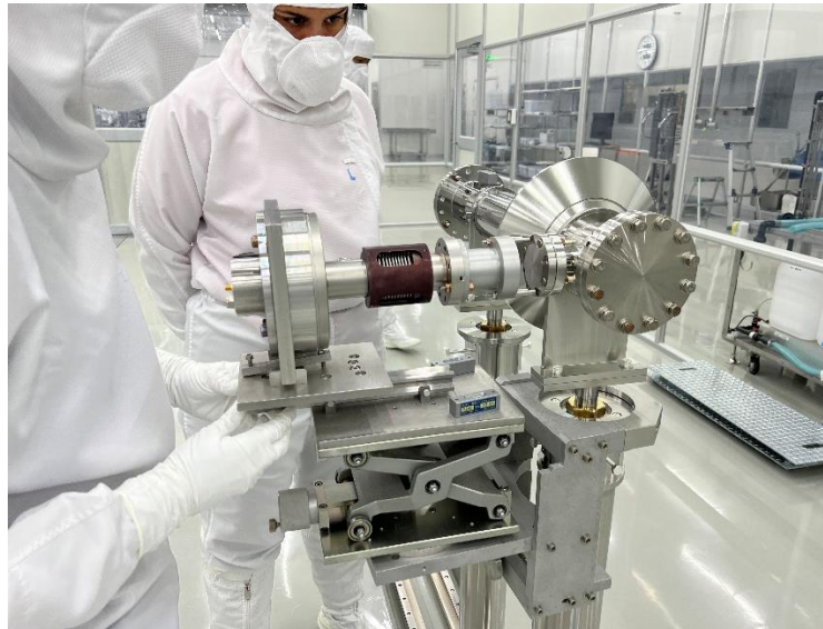
A demonstration of cold coupler installation using a mock-up cavity
