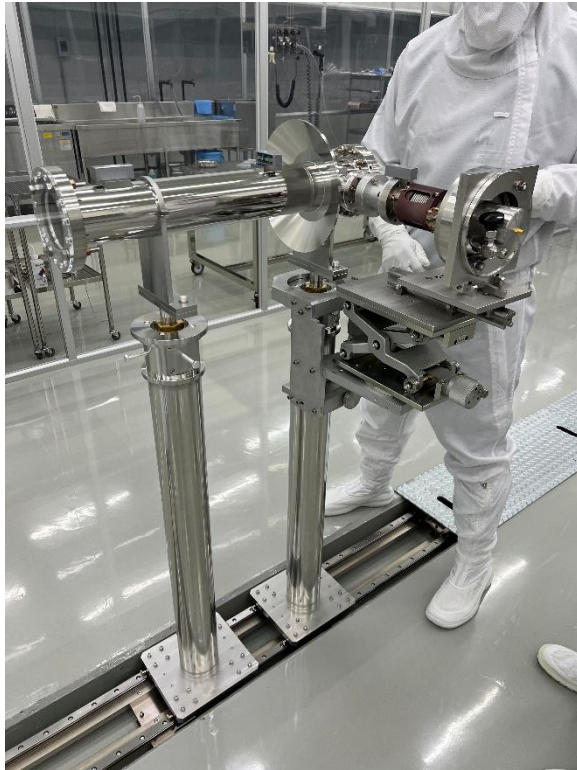
E-XFEL-type cavity support posts and coupler mounting jigs
