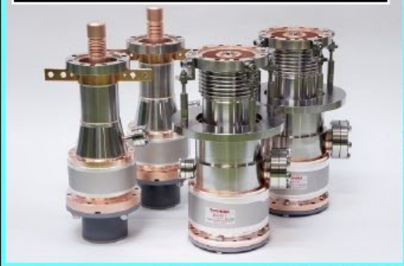
Power coupler (Copper plating on SUS316L)
