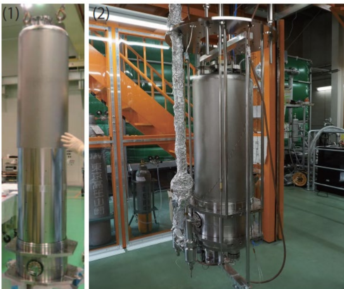
Figure 9: Photos of jacketed cavity: (1) Pre-assembly and (2) Assembly #3 prepared for VT
