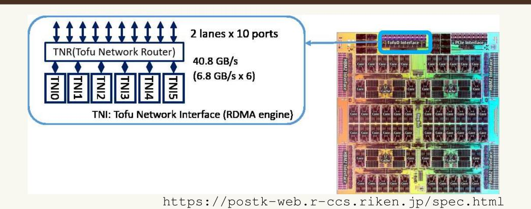
Flops/node: 3TFlops[double] (×23 of K-computer) injection BW/node 40.8GB/s (only ×2 of K-computer) communication is important
