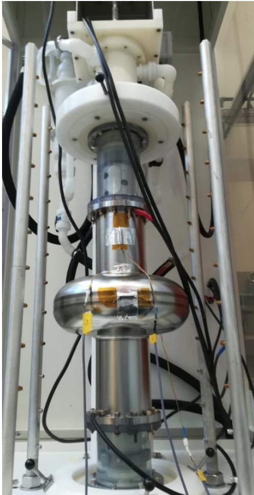
ESS 1C cavity on VEP set-up
