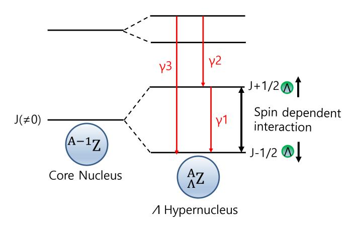
$\rightarrow$  By measuring energies of the  $\gamma$  rays, the split energy spacing is precisely estimated and we can know a fine structure of the hypernucleus.
