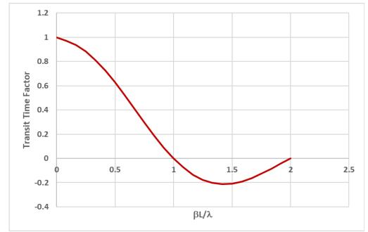
As seen  $V_0$  is the voltage gain of a particle passing through a constant DC field equal in the gap at time t = 0. The value of average field  $E_0$  depends on length L.
