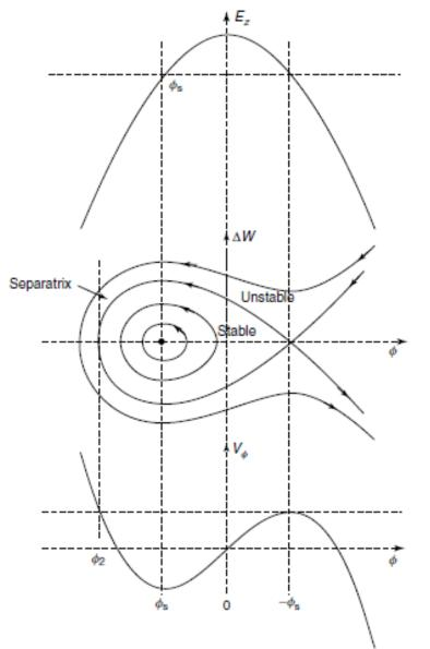
Accelerating field as function of phase. Note synchronous phase  $\varphi_s$  is negative
