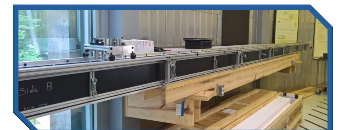
Dicounter dark box with the Cs-137 source on a moveable cart.
