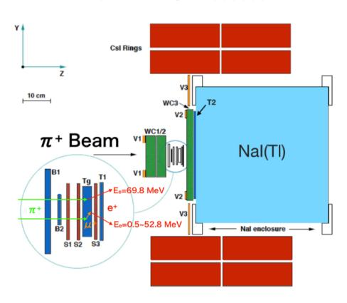
WC1-3 are wire chambers, S1-3 are silicon strips, and B1, B2, B3, T1, T2, V1, V2, and V3 are plastic scintillators (<u>Nucl. Instrum. Meth.</u> A791. 38-46(2015)).
