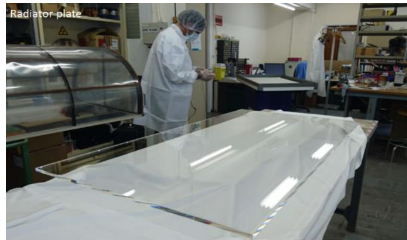
Quartz plate for prototype at CERN (half height w.r.t. LHCb requirements)
