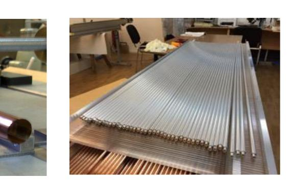
New adhesion style developed by JINR group for NA62 exp. at CERN, which was enabled by ultrasonic welding method, was adopted for COMET.
