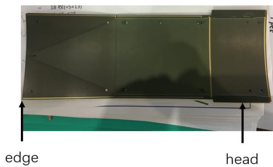
Figure 16: FPC Board. There are two different measuring position “edge” and “head” in the second measurement.
