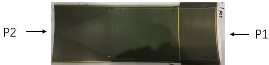
Figure 17: FPC Board. There are two different measuring position “P1” and “P2” in the third measurement.
